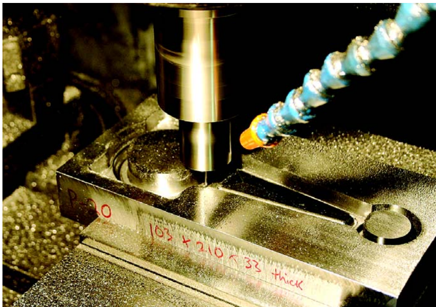
Direct machining of hard materials such as P20 reduces throughput time compared to EDM.
