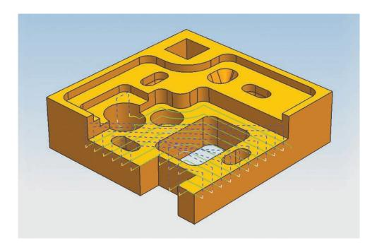
Face milling Solids-based face milling automatically respects part and fixture boundaries while efficiently clearing faces.
