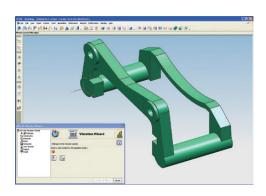
analysis processes. For each solid body component, users are prompted to assign a material specification, constrain the part, apply a load, automatically mesh the 3D geometry, and run the analysis using NX Nastran® software. With the NX Stress Wizard, users can review the structural performance image to ensure that the yield
