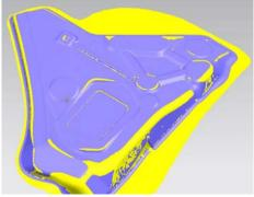
Example: Purple surfaces have to be morphed, according to the deviations seen in the yellow scanned mesh.
